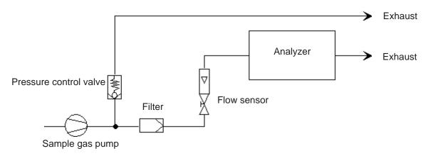
Fig. 4-3: Installation in bypass mode
